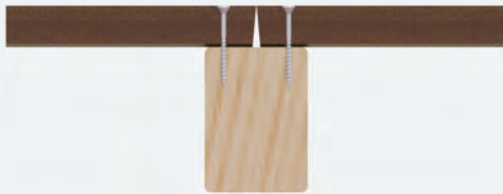
Slightly undercut for tight jointing
